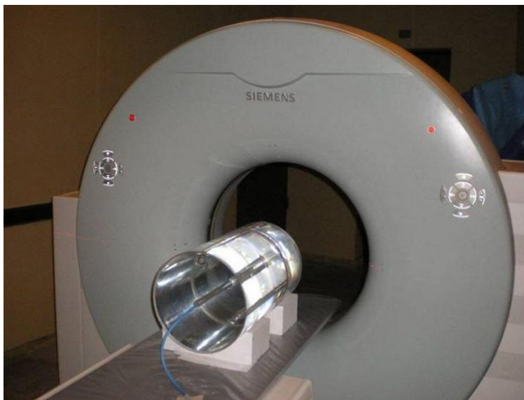
FIG. 1. Water phantom with the ionization chamber placed in the central insert.
