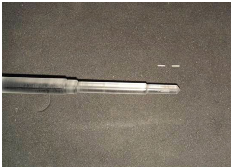
FIG. 4. TLD rod and insert to realize measurements in the water phantom.
